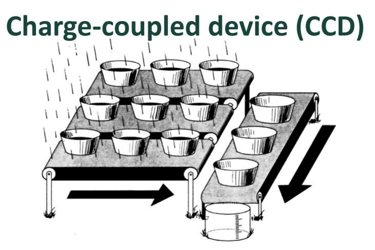
Fig. 2.1. CCDs can be likened to an array of buckets that are placed in a field and collect water during a rainstorm. After the storm, each bucket is moved along conveyor belts until it reaches a metering station. The water collected in each field bucket is then emptied into the metering bucket within which it can be measured. From Janesick & Blouke (1987).
