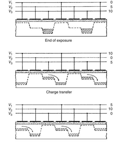
Fig. 2.2. Schematic voltage operation of a typical three-phase CCD. The clock voltages are shown at three times during the readout process, indicating their clock cycle of 0, 10, and 5 volts. One clock cycle causes the stored charge within a pixel to be transferred to its neighboring pixel. CCD readout continues until all the pixels have had their charge transferred completely out of the array and through the A/D converter. From Walker (1987).
